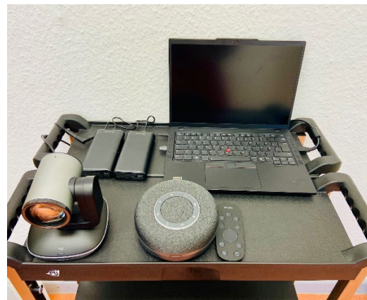
Fig. 5: Setting up a PTZ system on a mobile table.
