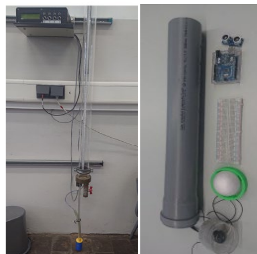
Figure 4: Original control loop experiment (submersible pump) (left) and components of the first prototype control loop for Praktika@Home (right) [5]
