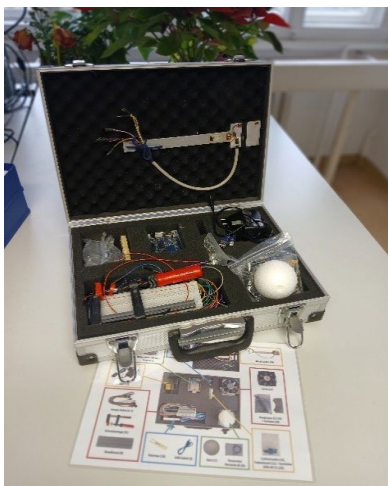
Figure 3: Experiment kit with the Arduino, sensors, actuators, and cables (current contents)
