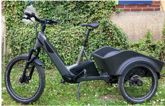
Fig. 7: The chair's cargo bike as the basis for installing the hydraulic drive.
