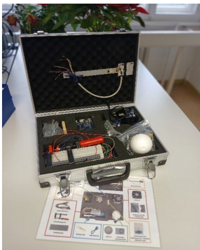
Figure 3: Experiment kit with the Arduino, sensors, actuators, and cables (current contents)
